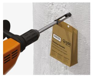
3. Drill to 9 cm, remove while the drill is rotating at low speed.
