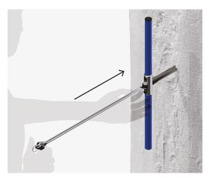
6. Rotate handle 720° anticlockwise to detach core.
