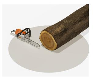
3. Keep the chainsaw close to the ground when cutting.
